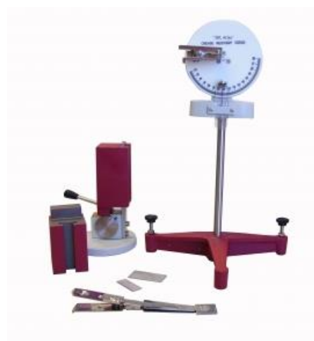
84-rasm. M003A SHIRLEY CREASE RECOVERY TESTER & LOADING DEVICE asbobi.
