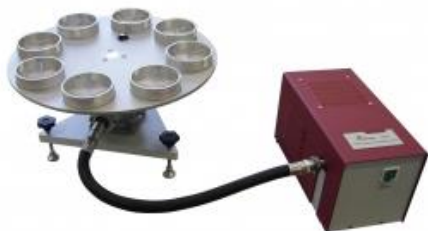
91-rasm. M261 Water Vapor Permeability Tester asbobi.
