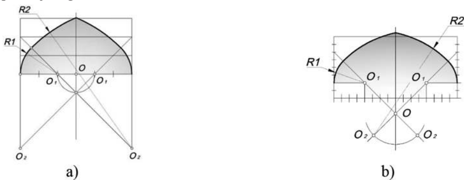
2-rasm. To‘rt markazli arkalarning geometrik yasalishi.
