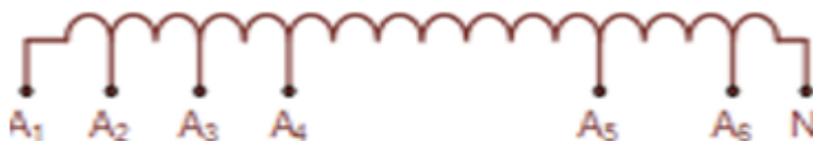
3.14-rasm. Avtotransformator chizmasi
