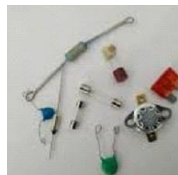
8.12-rasm. Eruvchan saqlagich
