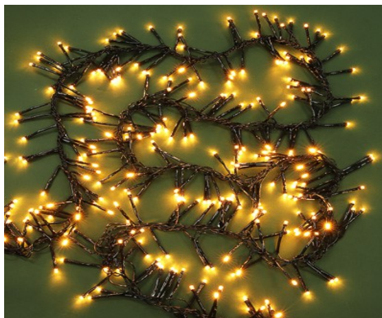
4.2-rasm. Yangi yil archasini bezatish uchun ketma-ket ulangan yorug‘lik diodlari
