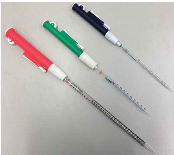
Figure 1.1 Serological pipettes and pumps for total volumes of 25 ml (red pump), 10 ml (green pump), and 5 ml (blue pump).
