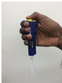
Figure 1.3 (a) Up position of the plunger button on a micropipette. This is the starting position for proper pipetting. (b) The plunger button is depressed to the first stop position to initiate pipetting. While holding the plunger button in this position, insert the micropipette tip into the sample and then slowly release the plunger button to the up position. The desired volume of sample will be drawn up into the tip. (c) When the plunger button is depressed beyond the first stop position to the second stop position, the liquid in the pipettor tip will be completely expelled.
