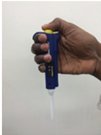
Figure 1.3 (a) Up position of the plunger button on a micropipette. This is the starting position for proper pipetting. (b) The plunger button is depressed to the first stop position to initiate pipetting. While holding the plunger button in this position, insert the micropipette tip into the sample and then slowly release the plunger button to the up position. The desired volume of sample will be drawn up into the tip. (c) When the plunger button is depressed beyond the first stop position to the second stop position, the liquid in the pipettor tip will be completely expelled. (See insert for color representation of the figure. )
